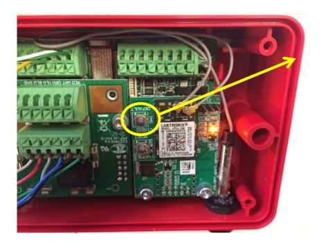
TIP when needed – you can use the <u>default button for</u> a total reset of the unit (press and hold for more than 6 s.)
