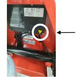
2. Plug the USB charger into an outlet and the device will start charging (a **red** light is shown around the charging plug).
