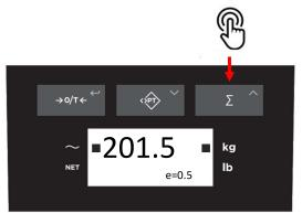
The total weight and the amount of weighings is shown in the bottom-left corner of the screen.
