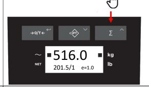
The weight has been added to the total and the weighing counter has been increased. The total weight will follow the highest weighing graduation.
