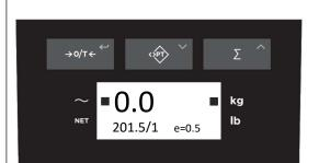
With a new load press the totalise button again to add the weight to the total.
