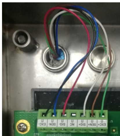
Figure 4-3: Analog Load Cell Connection Terminal
