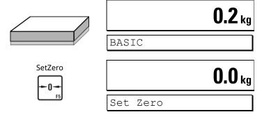
Set gross weight to zero (only within selected range for pushbutton zero).
