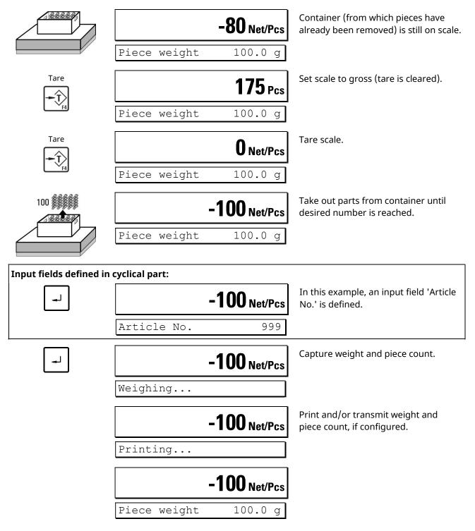
Take out further parts or remove container from scale.
