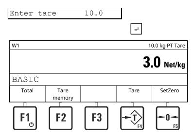
**Note:** Enter '0' and confirm with tare key **F4** to clear the set tare value. Subsequently the weight display shows the gross weight.
