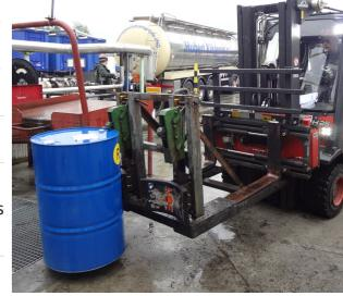
substances are used in some areas, some of the mobile weighing systems are also ATEX explosion proof.
