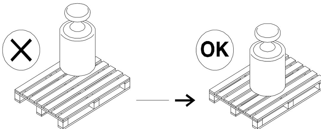
The iJack comes equipped with a level switch. This means that when the system is tilted by greater than  $2^\circ$  the indicator will automatically shut off. An uneven floor will have a greater effect on weighing ability. An even floor is optimal.
