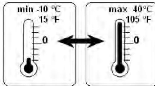
Temperature range: between 15 – 105 °F (-10 - +40 °C) the maximum inaccuracy is 0.1% of the weighed load. Outside this range inaccuracies of up to 0.3% may occur.
