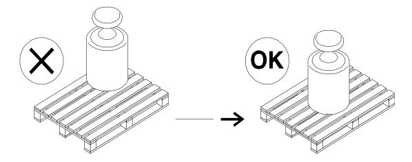
The iJack comes equipped with a level switch. This means that when the system is tilted by greater than 2° the indicator will automatically shut off. An uneven floor will have a greater effect on weighing ability. An even floor is optimal.
